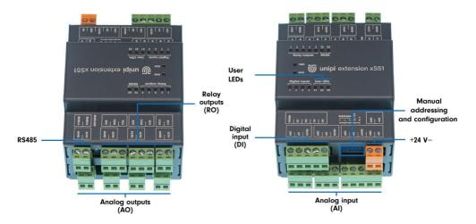
The number and position of I/O can vary for a particular unit (see <u>Unipi Knowledge Base</u> for details).
