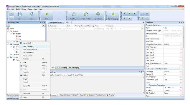
In solution explorer, under the PLC icon, you will find a newly created channel. Select that channel by left clicking on it and in the right part of the screen you will see its <u>properties</u>. Set is as following:
