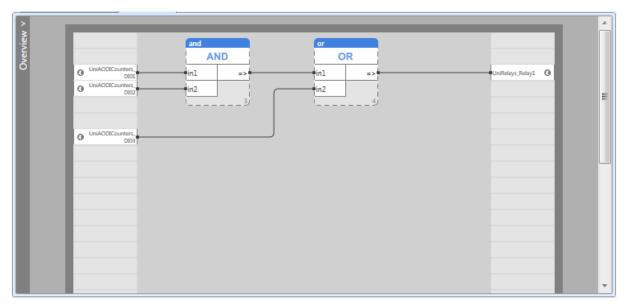
After finishing all the steps above, <u>Build solution</u> (Ctrl+Shift+B) and check for any errors or warnings, which can be seen in the Results tab at the bottom of the screen
