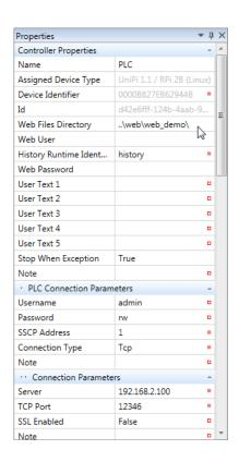
• Now left click on the PLC in Solution Explorer, and then click on <u>Upload web</u>. After the upload is done, you can open web browser and type the IP address of the UniPi as an URL address. You should see the web panel. If not, try refreshing the page or rebooting the UniPi.
