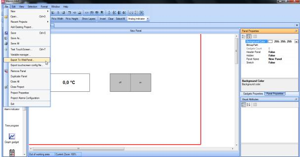
Now go to Mervis IDE and open the project. You have to add the exported project to the device configuration. In <u>Controller properties</u> locate <u>Web files directory</u> column, and add the path to the exported folder. You can also set up <u>Web user</u> and <u>Web password</u>, if you needrestrict access to control of the web panel
