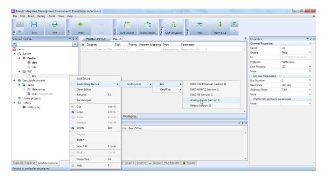
Because of being in Simple Mode, the Autogen feature automatically generates and maps variables to physical inputs and outputs.
