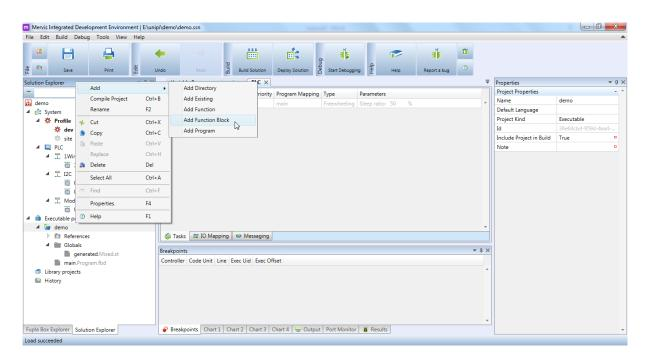
A new program appears in the Solution Explorer, double click on it to see the function block's structure. Type the following code to the editor:
