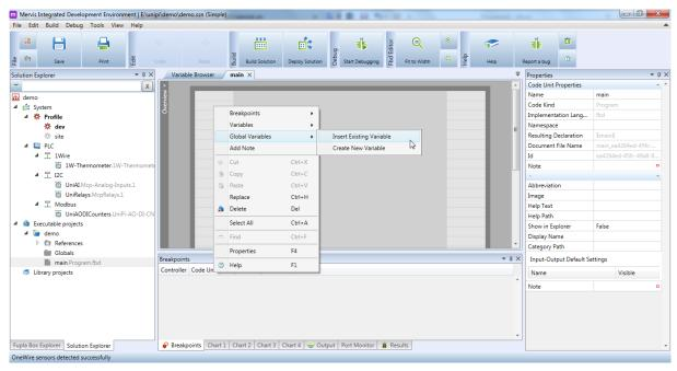
Then repeat the same process, but instead of adding a variable into the inputs column, add UniRelays Relay1 into the outputs column
